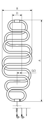
$A-Height\ B-Width\ C1-C5-Distance\ between\ pipe\ centres\ D-Horizontal\ distance\ between\ mounting\ bracket\ centres\ E-Vertical\ distance\ between\ mounting\ bracket\ F-Distance\ between\ a\ mounting\ bracket\ and\ the\ bottom\ of\ the\ radiator$
