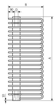
$A-Height\ B-Width\ C1-C5-Distance\ between\ pipe\ centres\ D-Horizontal\ distance\ between\ mounting\ bracket\ centres\ E-Vertical\ distance\ between\ mounting\ bracket\ F-Distance\ between\ a\ mounting\ bracket\ and\ the\ bottom\ of\ the\ radiator$
